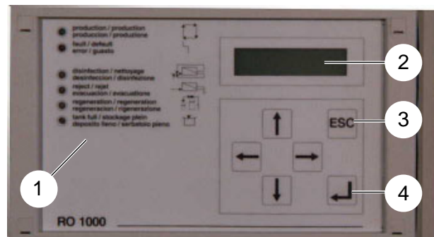
Figure 5 Control panel and display
